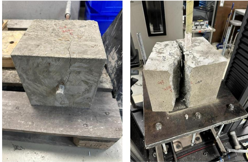
Figure 8. Representative post-test damage observed during the pull-out programme: (a) cracking radiating from the GFRP bar; (b) complete splitting of the concrete cube.
