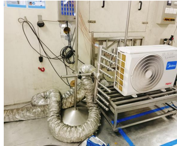
Figure 3. Psychrometric laboratory installation: outdoor-unit installation
