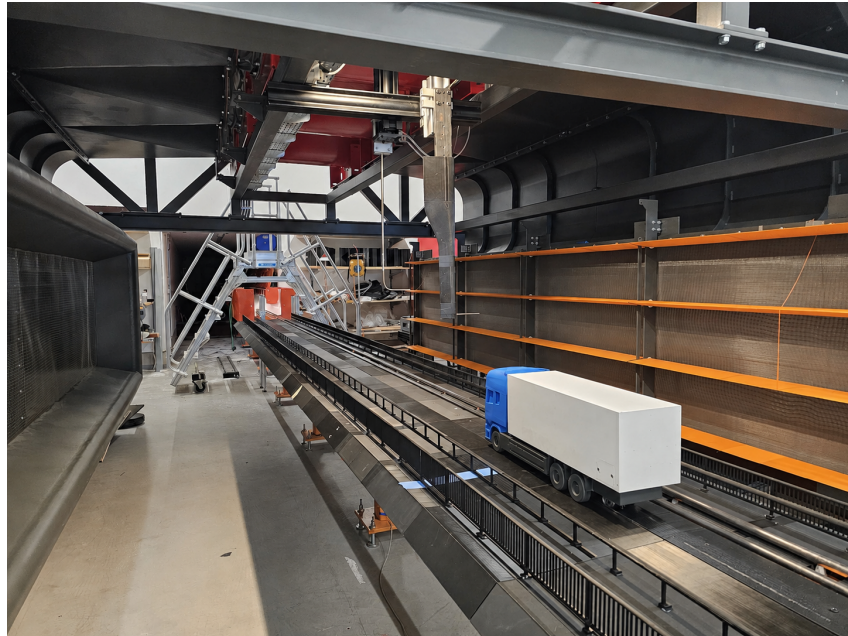
Figure 2. Image of the tunnel section with the bridge model installed in configuration (iii), the flap system seen on the right, and both the pitot-static tube and five-hole probe in the middle. Note: the truck model was added to this image from another similar image by OpenAI, ChatGPT , August 2026 ( https://chat.openai.com ).
