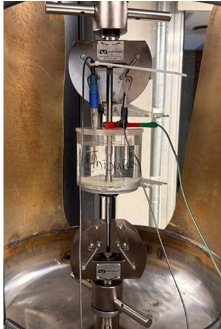
Figure 4. SSRT test setup with in-situ electrochemical hydrogen charging
