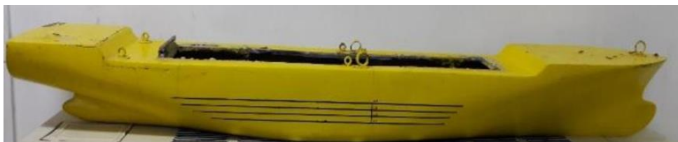
Figure 1. The model of the KCS ship that was tested in the towing tank [30].
